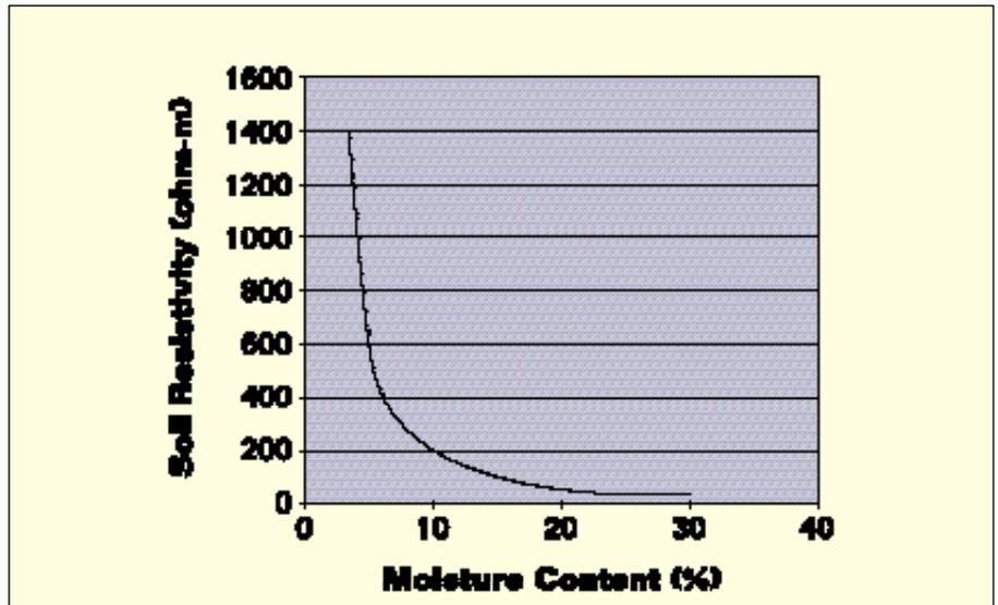
Figure 2 Soil Resistivity – Moisture Content
