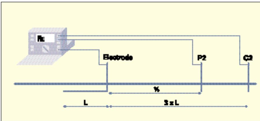
**Figure 4 Fall of Potential Testing**
